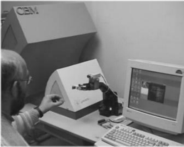
Fig. 2. Robotic arm controlled using a PPNN loaded into a dedicated hardware (CBM).
